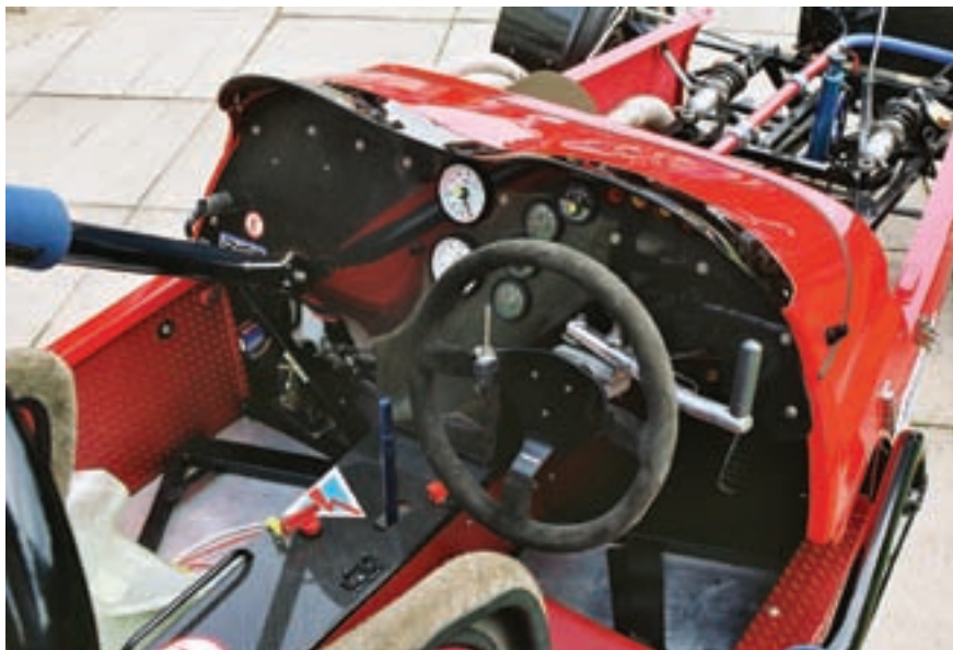
Above: The engine sits almost alongside the driver for optimum weight distribution. In the absence of a door, Chris has fitted a swing-up frame.
